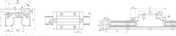
\*\*E: Size 15 delivered with straight standard nipple. Size 20 – 55 delivered with angled standard nipple.
