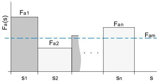
Diagrams presented above are showing theoretically determined service life of the ball screw when mean axial force  $F_{am}$  is taken into consideration.
